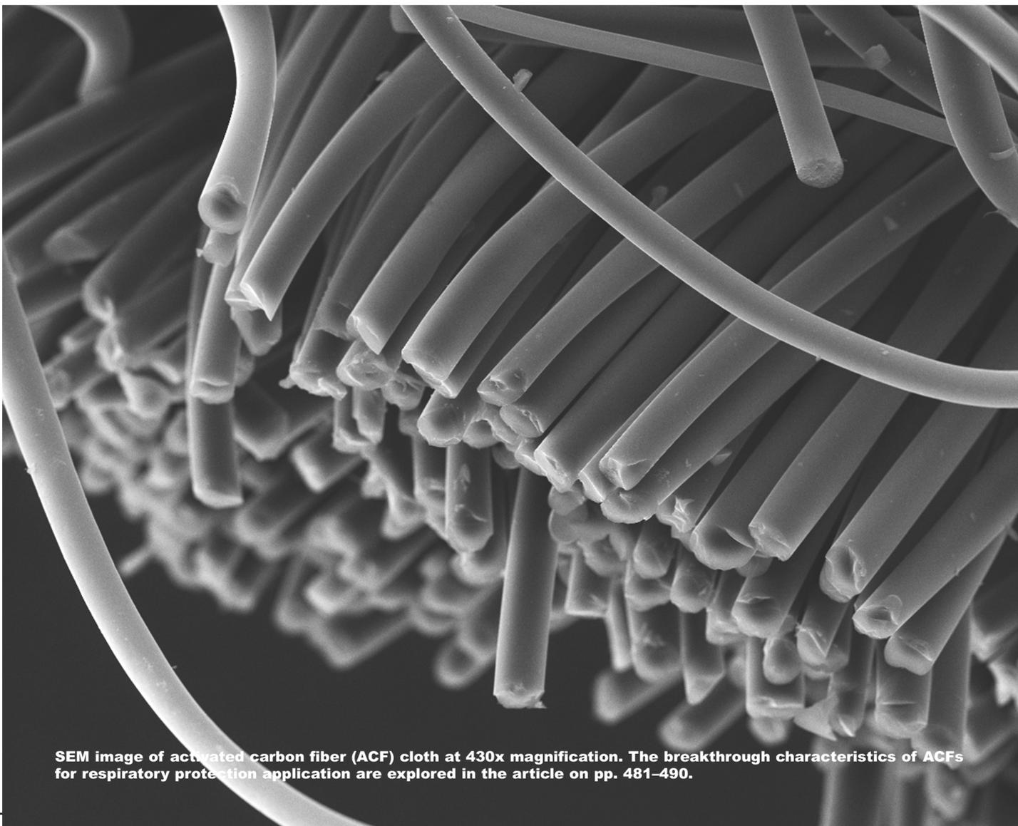
**SEM image of activated carbon fiber (ACF) cloth at 430x magnification. The breakthrough characteristics of ACFs for respiratory protection application are explored in the article on pp. 481-490.**
