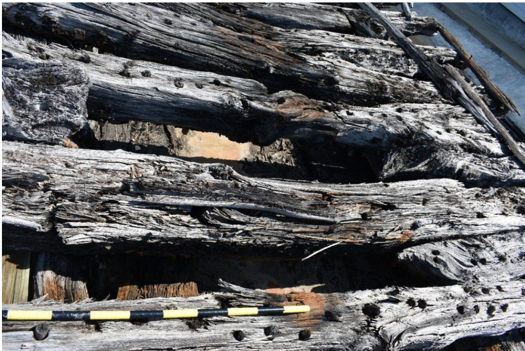
Figure 24. Frames showing bleaching, drying and severe degradation (Photo credit: Tyler Ball, ECU)
