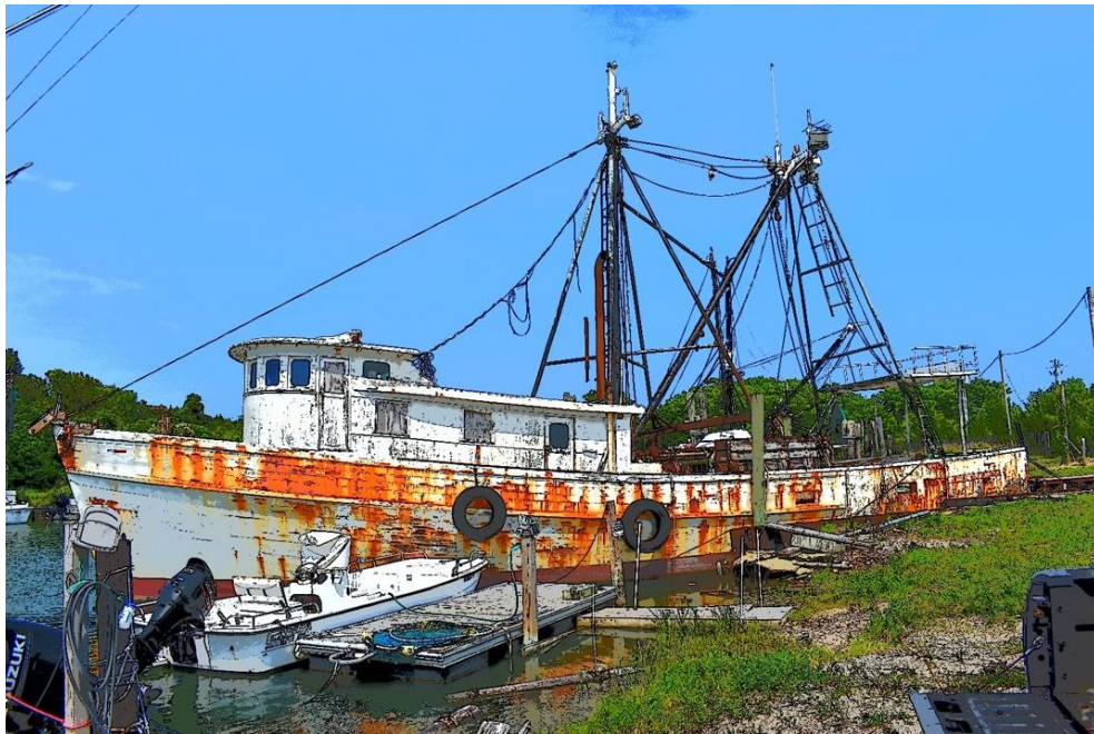
Figure 151. Derelict locally-built 70-foot shrimp fishing boat Lady Barbara profile view (Photo by Lynn Harris, ECU).
