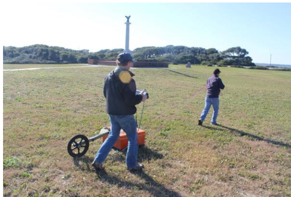
Figure 7. David Mallinson (left) and Barry Bleichner (right) deploying the ground penetrating radar unit at Fort Fisher historic battle field (Photo by Lynn Harris).
