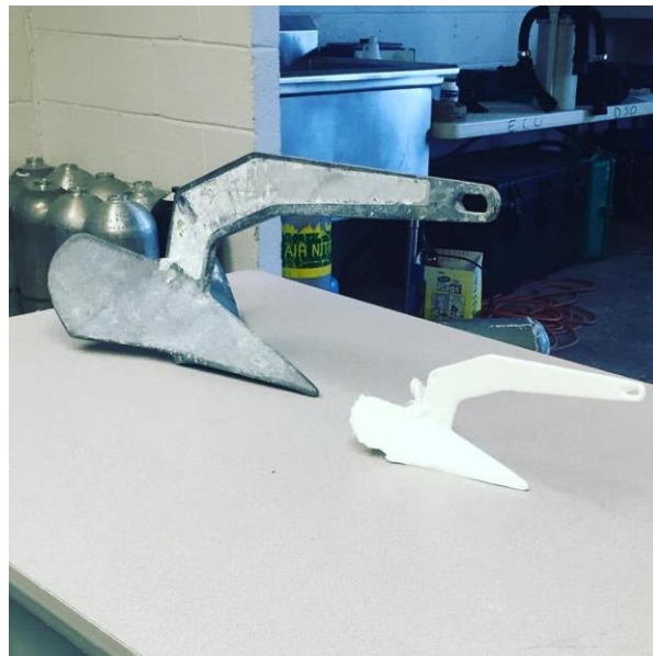
Figure 6. A 3D Printed anchor created by student Annie Wright using underwater photogrammetry (Photo by Lynn Harris).
