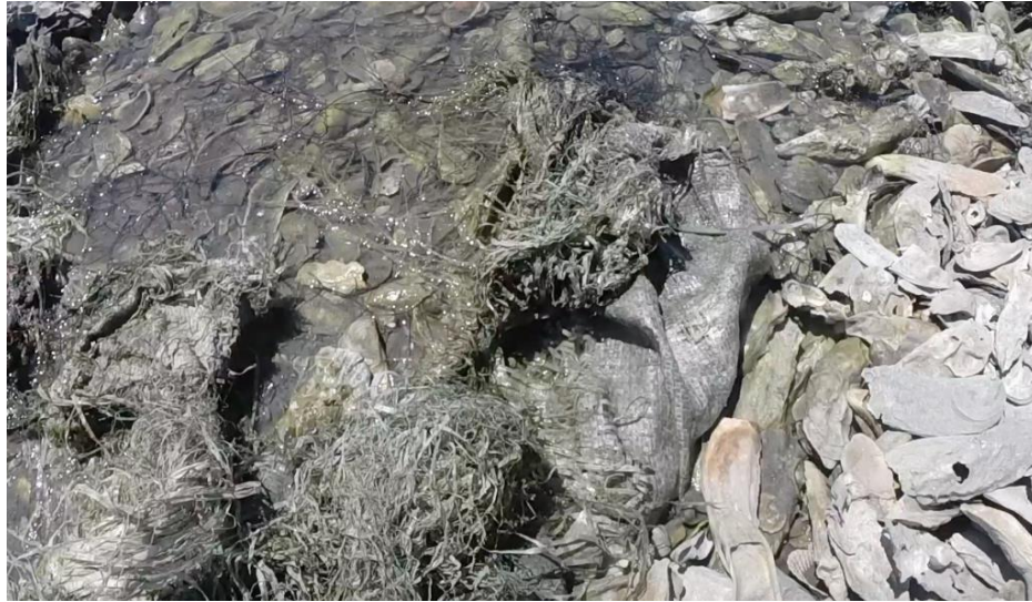
Figure 43. Stabilizing sandbags on the site shredding and eroding (Photo by Jeremy Borrelli).
