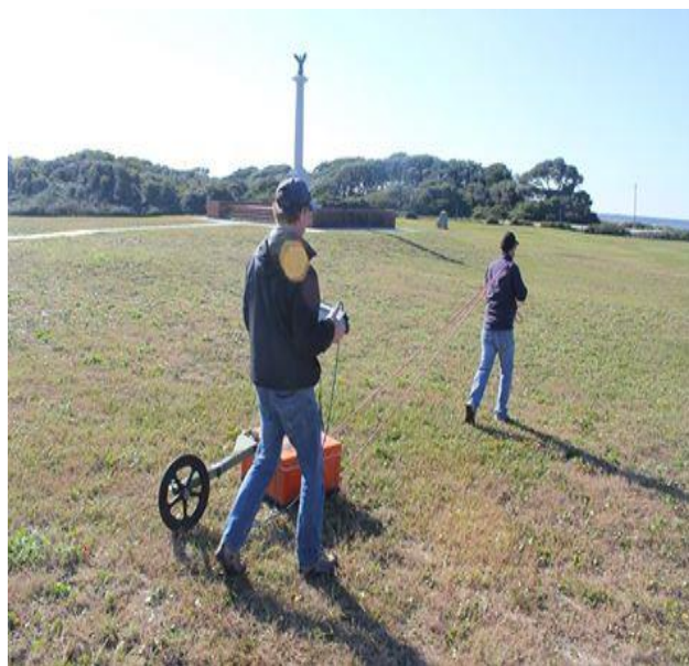
Figure 19. Geology team conducting Ground Penetrating Radar operations at Fort Fisher (Photo by Lynn Harris)
