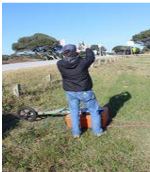
Figure 19. Geology team conducting Ground Penetrating Radar operations at Fort Fisher (Photo by Lynn Harris)
