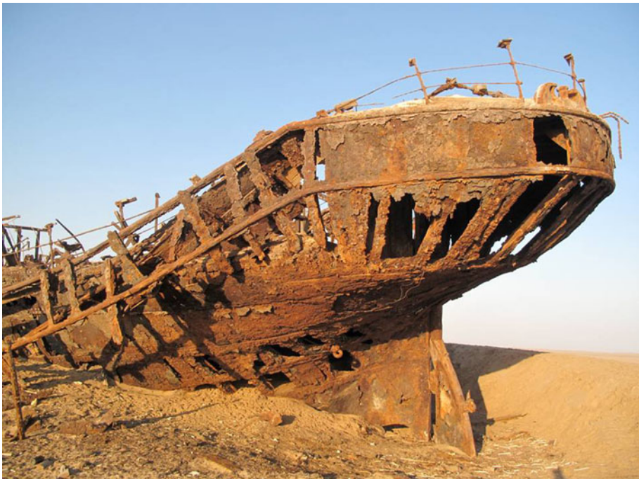
Fig. 12 Eduard Bohlen II stern port view of collapsed guard rail and rudder (WUC photograph)
