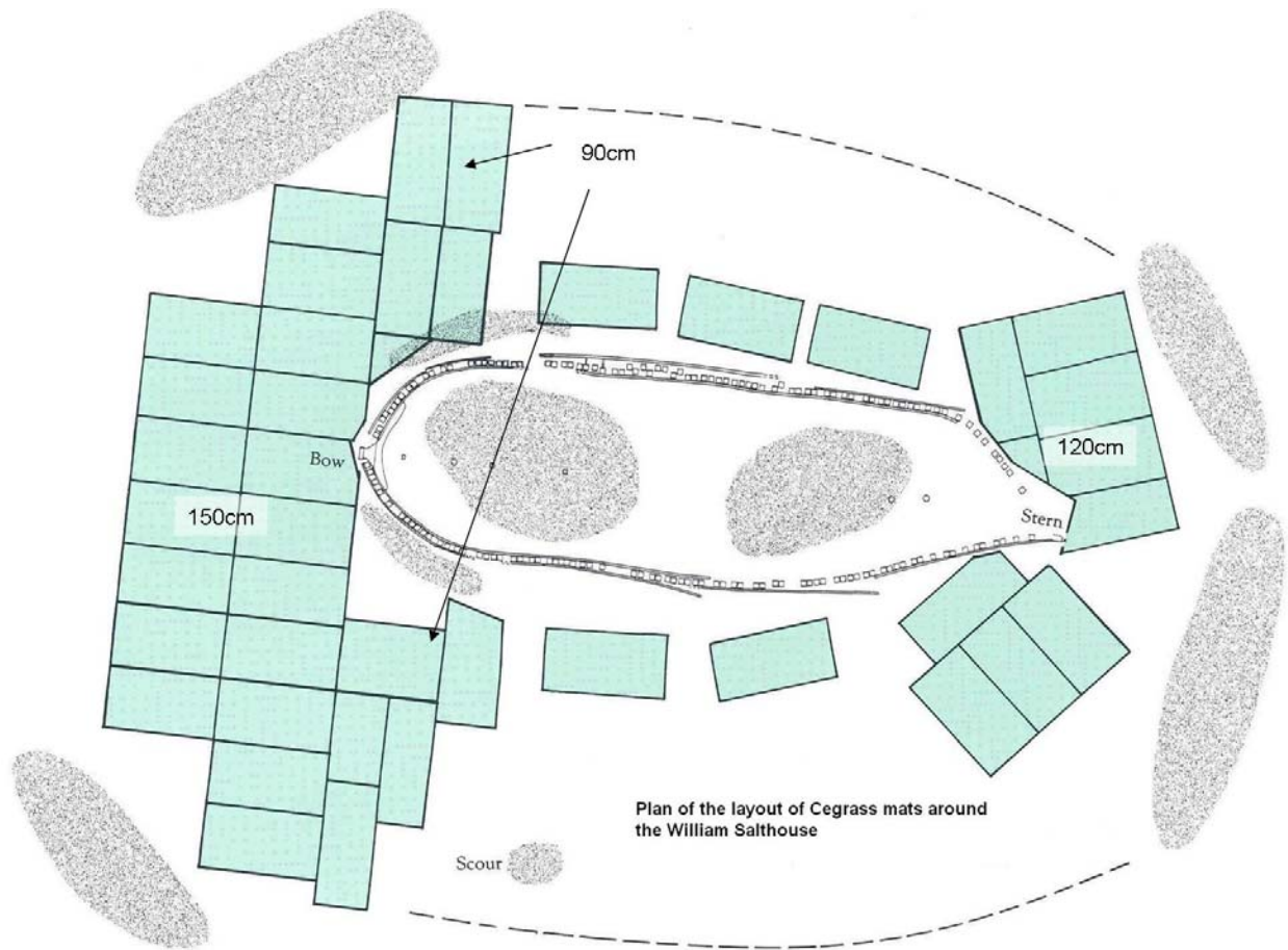
Figure 4-5 Position of the Cegrass™ mats around the William Salthouse wreck (Heritage Victoria 1990).
