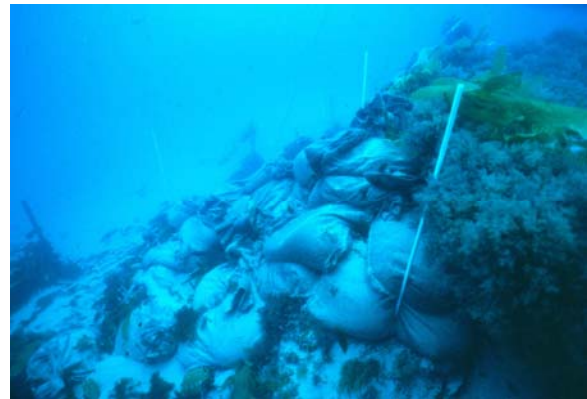
Figure 4-3 Sandbags on the William Salthouse wreck supporting the hull structure (Heritage Victoria 1988).
