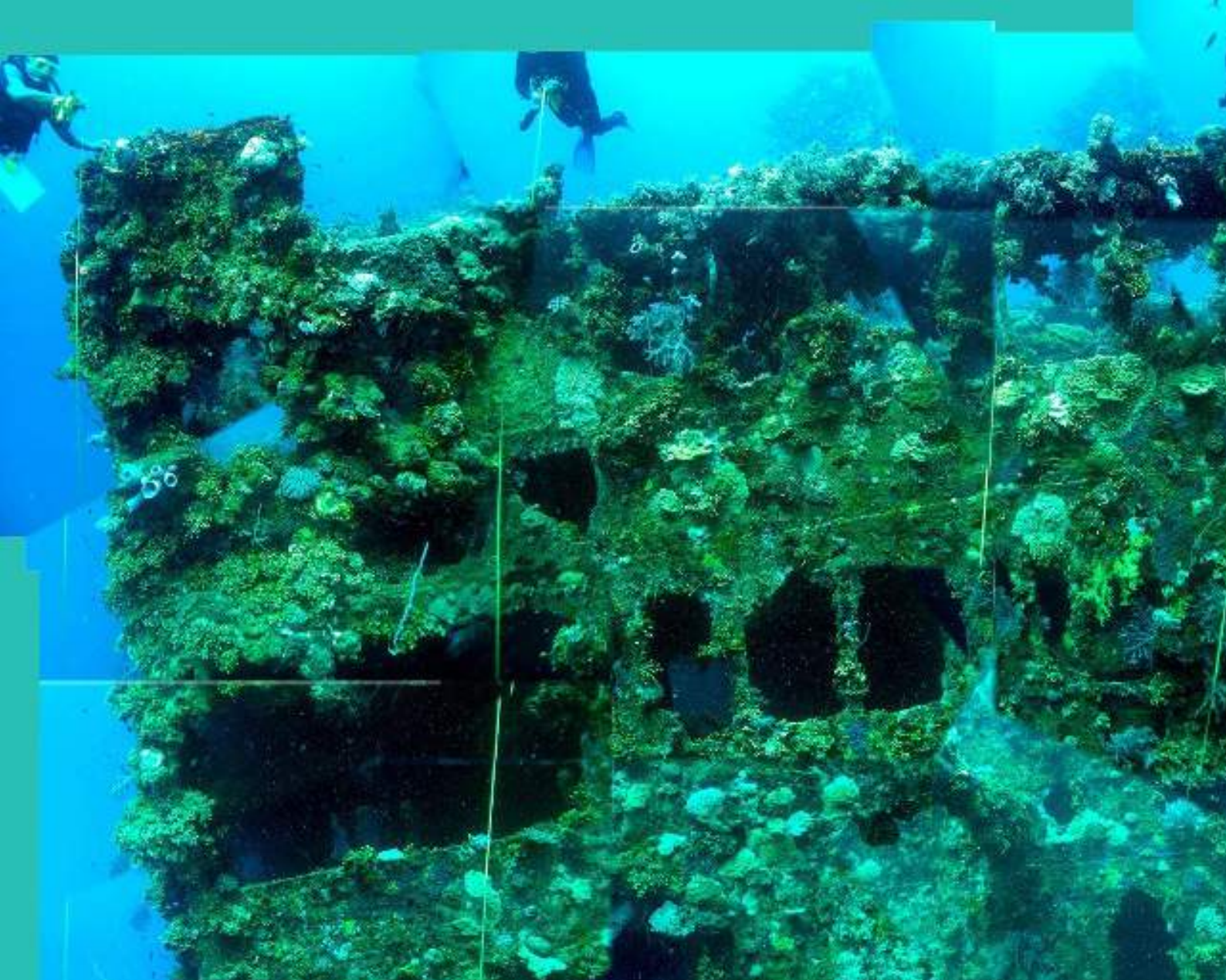
Figure 5-5. Photo-mosaic of the bridge face of Fujikawa Maru showing the impact of dynamite fishing. This area should be totally covered with corals and sponges but many have been killed by dynamite fishing which also greatly weakens the iron structure and renews corrosion. In 2012, Dianne Strong, a frequent visitor to Chuuk reported that the bridge collapsed in the middle. ©Bill Jeffery 2006
