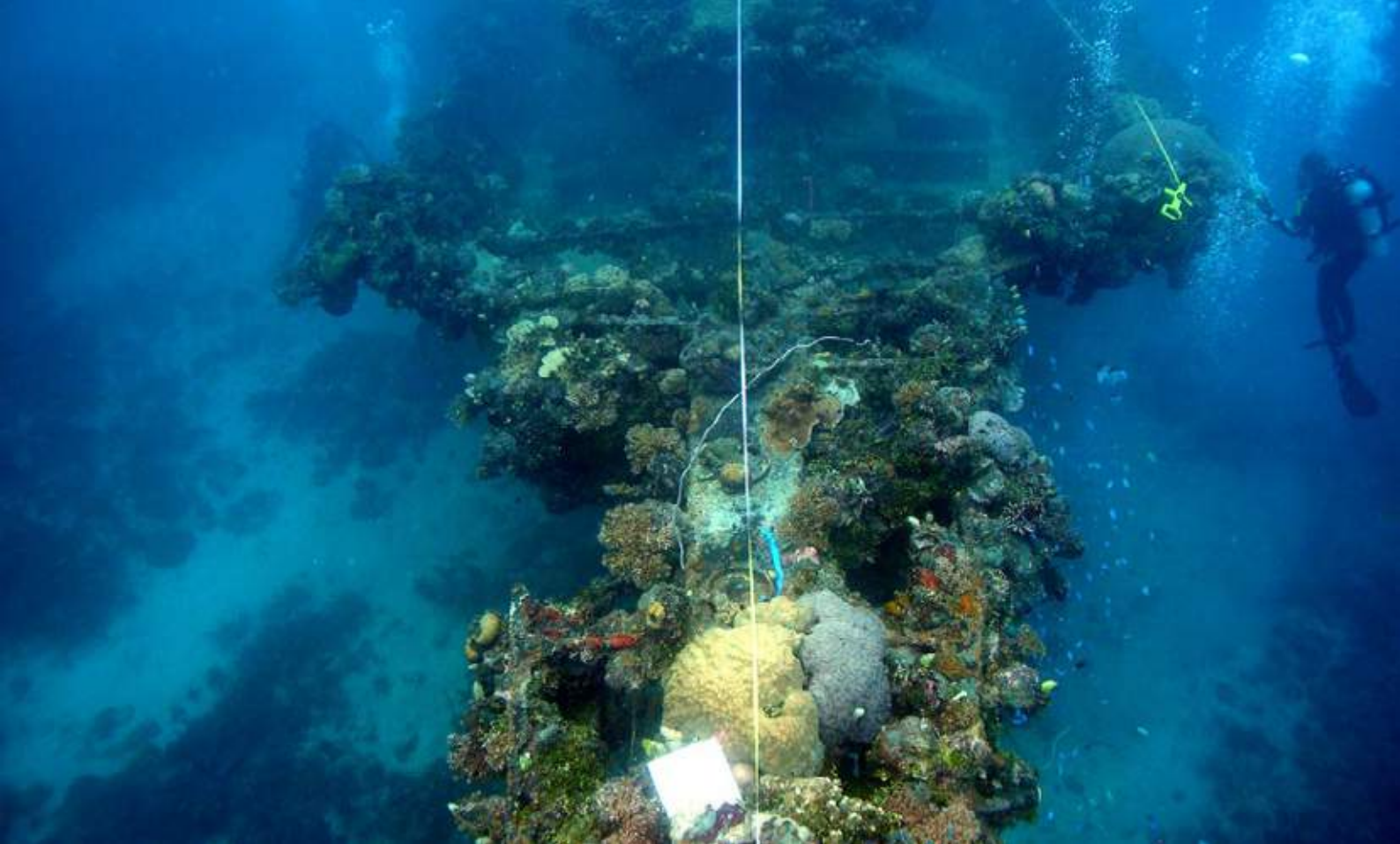
Figure 5-9. The bow showing the bowsprit, sponsons on the port side and the bandstand on 'Unknown G' site. ©Bill Jeffery, 2006
