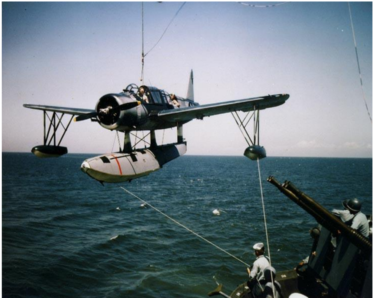
Figure 82. The Vought OS2U Kingfisher Aircraft as Configured for Sea Launch and Recovery. (Source: National Archives).
