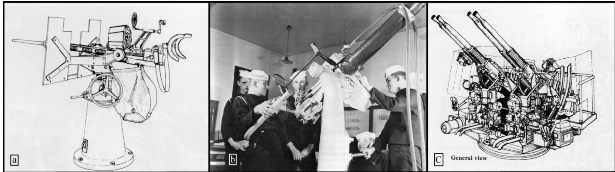
Figure 80. Images of the three types of machine guns used aboard the ships in Escort Group Easy. 5.19a is the 20mm Oerlikon, 5.19b is the Browning M2, and 5.19c is the 40mm Bofors. (Source Campbell 1985:148-153; Friedman 1988:75-79).
