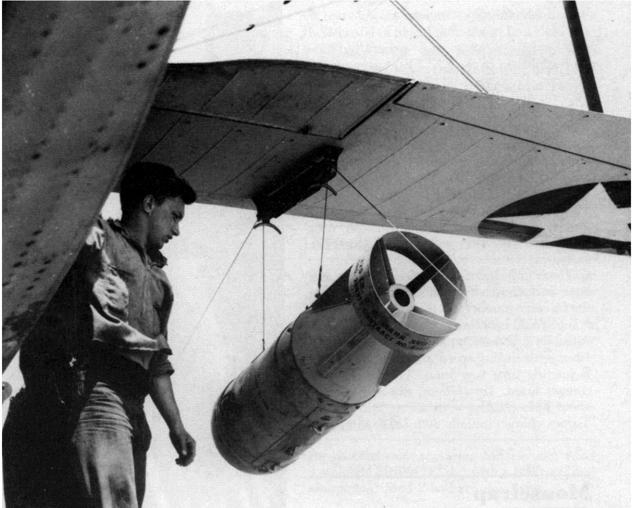
Figure 83. A Mk 17 aerial depth charge being unloaded from a patrol aircraft. (Source Campbell 1985:165).
