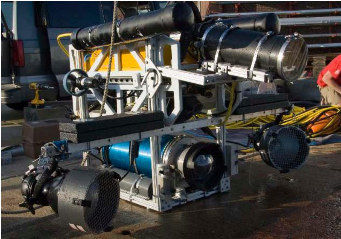
FIGURE 12. Modified Stingray ROV system with a 3D visualization payload (Image: WHOI:AIVL).
