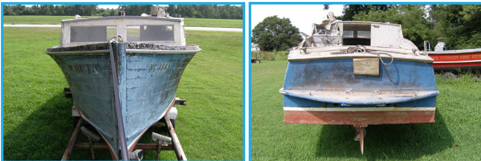
Three views of NCHH0025 with noted dead-rise and bow flair, Currituck, NC (Photographs by Brian Diveley, 2005)
